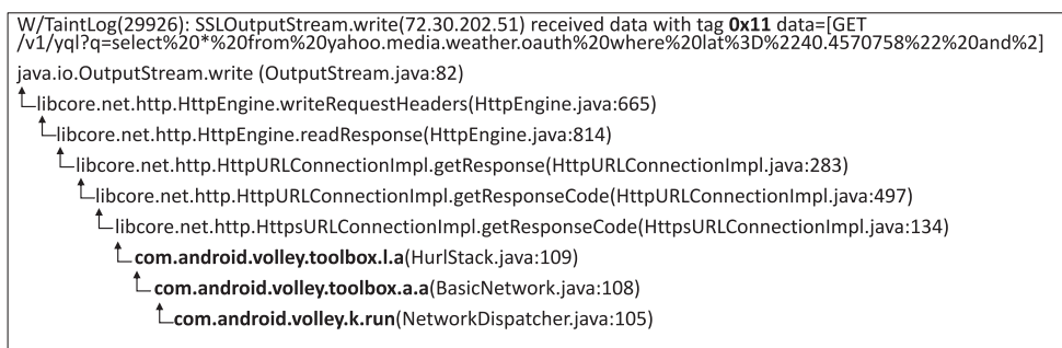
Fig. 4. An example call stack from the Yahoo Weather app showing the challenge of stack traces with multithreading. The app tried to send location data (tag 0x11) to a remote server. However, due to a common design pattern, when we get the call stack at a taint sink, we only get it from the current child thread. As a result, a great deal of potentially useful information has been lost.
